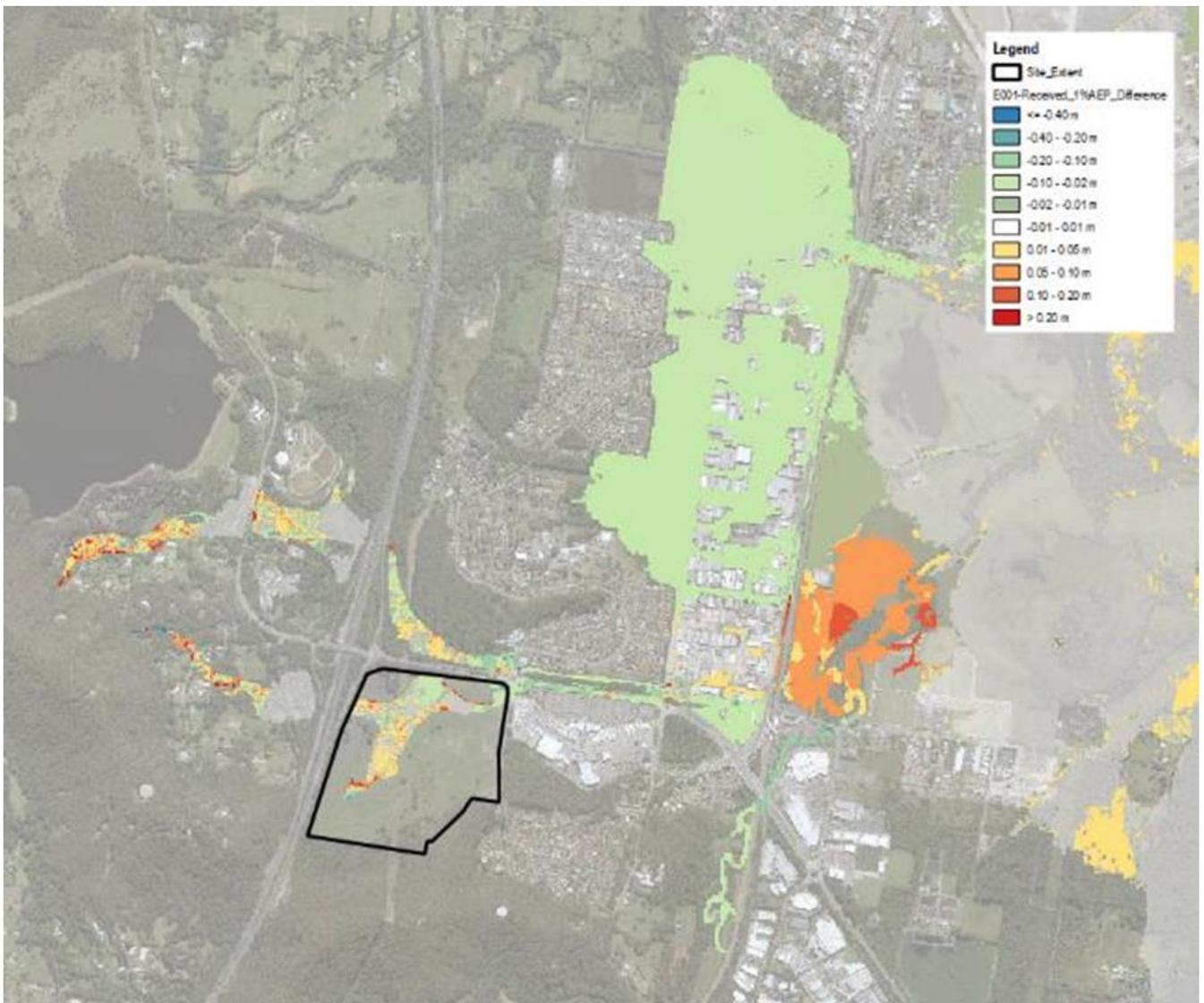
Figure 4-1 Stantec base case – provided 1% AEP WSL difference
