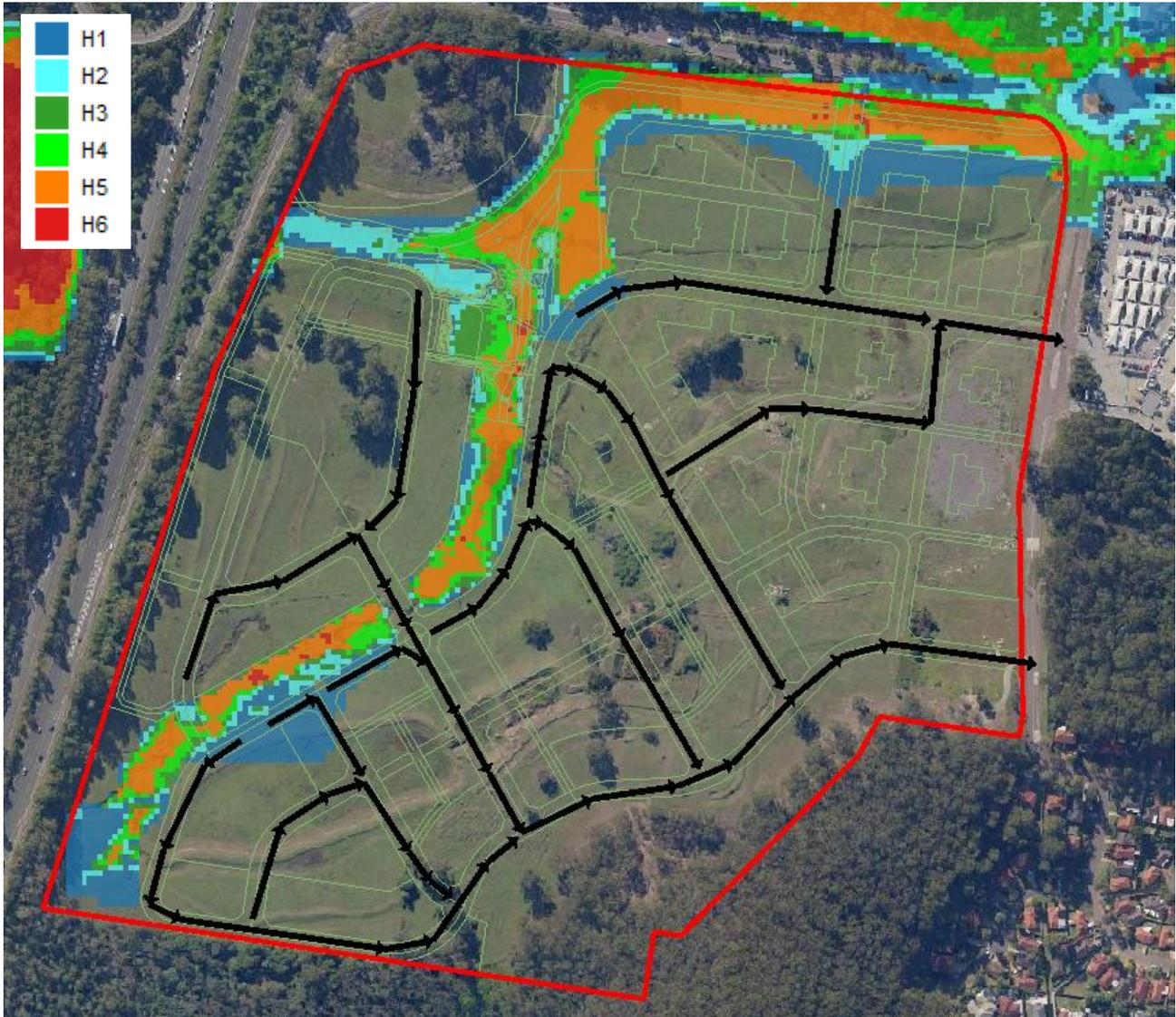
Figure 5-2 Proposed PMF immune access and evacuation (evacuation route: black arrow, PMF Hazard: background)
